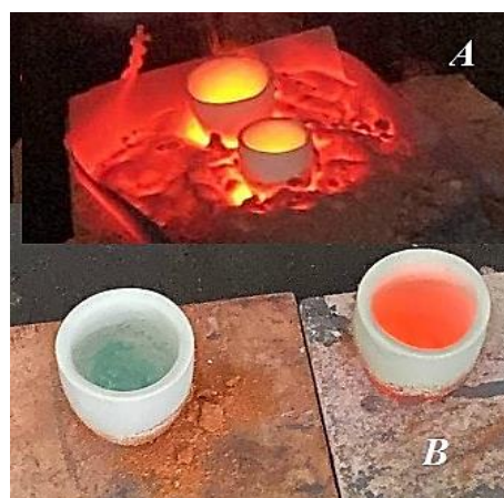
Figure 1 – Photo of the charge sintering process (A) and the finished product after drying (B)
