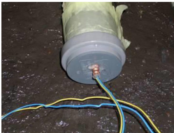
Fig. 3. Method of firing of the MWE type RP charge
