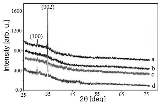
Fig.1. X- Ray diffraction , pure ZnO films and ZnO film doped with Al, (1, 3, and 5 %) (a,b,c,d)
