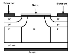
Fig. 1 – Schematic design of Superjunction MOSFET. Structure shown represents one cell of the device
