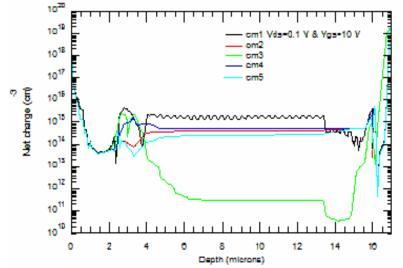
Fig. 6 – Comparison of net charge in the on-state w.r.t. the variation in the pillar width
