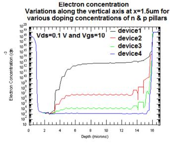
Fig. 5 – Electron concentration variations in the on-state
