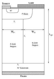
Fig. 2 – Cross section of a SJ MOSFET
