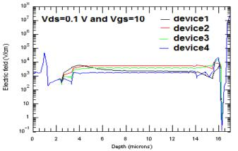
Fig. 4 - Electric field variations in the on-state for various devices
