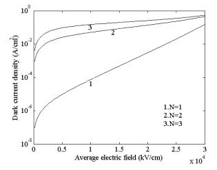
Fig. 1 – Variation of dark current density with electric field
